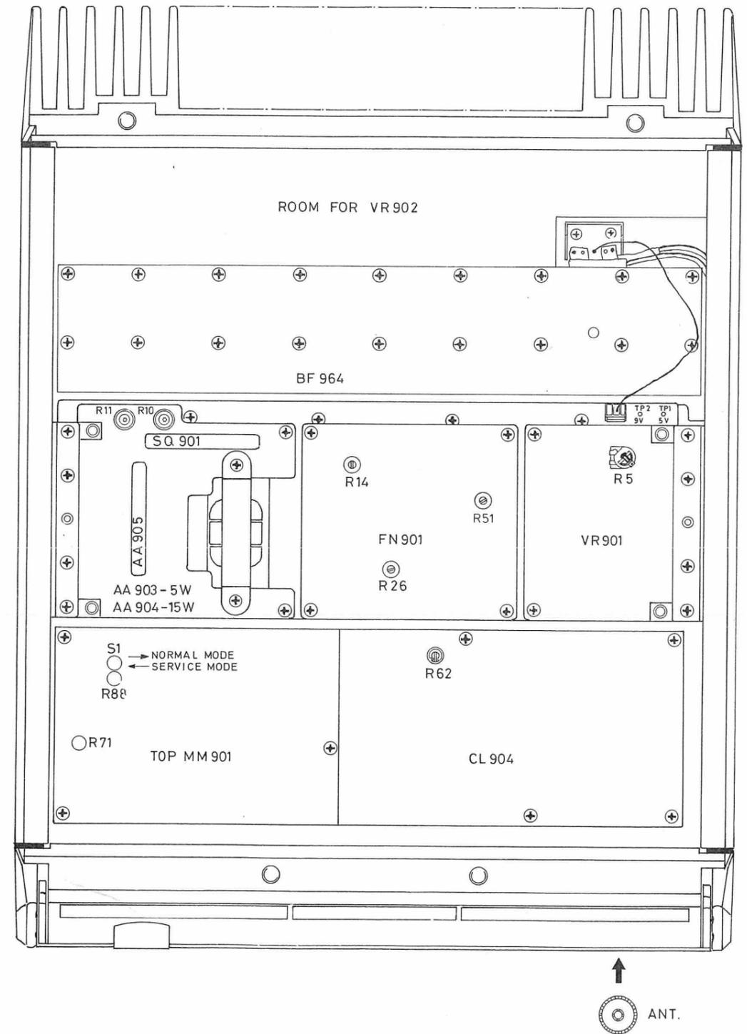
ADJUSTABLE COMPONENTS AND MODULE LAYOUT
