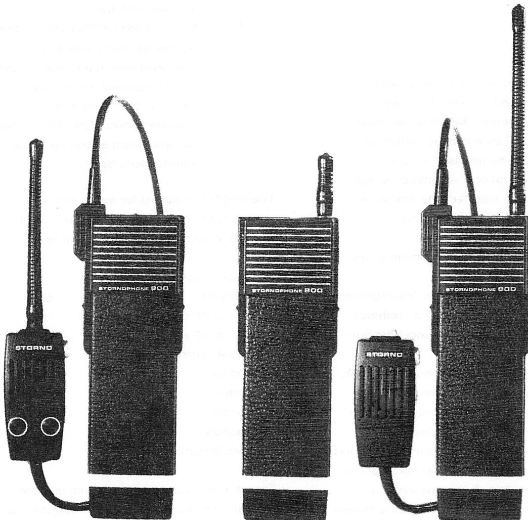
The STORNOPHONE 800U portable radiotelephone is a universal combination transmitter and receiver for FM radio communication service on fixed, crystal controlled frequencies.
