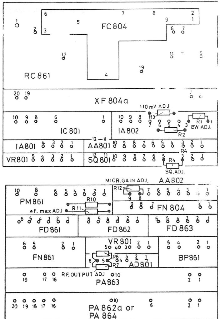
Fig. 8. TERMINAL LAYOUT CQP864U
