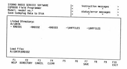
To specify the directory path and file name for the save file, follow the procedure described in section 8.2.2 for loading data files. The exception to the procedure is that you must press the F6 key (instead of F7). Once you have specified the filename, press ENTER. If the filename already exists in the current directory you will be given the warning:
